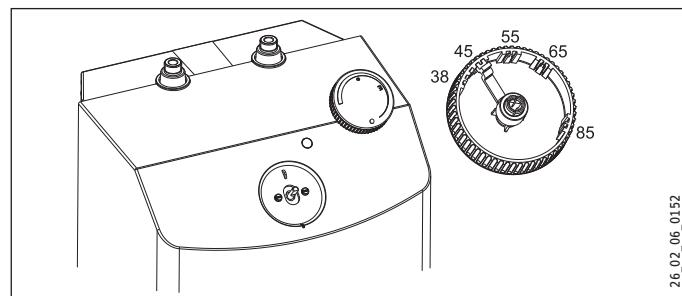
The lever underneath the temperature selector allows you to limit the setting range of the temperature selector to a specific maximum temperature.
